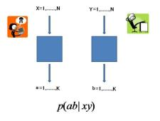
Figure: Alice and Bob measurements. Inputs: x and y, Outputs: a and b. P(a, b|x, y) is the probability of obtaining the pair (a, b) when Alice and Bob measure, respectively, with the input x and y.
